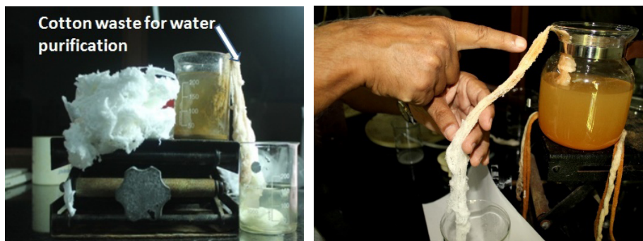
SF1. Cotton waste for water purification. Suspended impurities are held in the beginning of the filtration.
